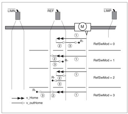
Figure 8.5 Reference movement to reference switch
