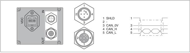
Figure 6.14 Pin assignment of CAN fieldbus interface
