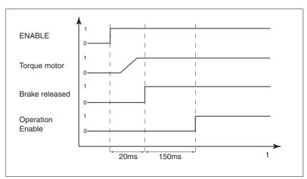
Figure 8.8 Releasing the holding brake
