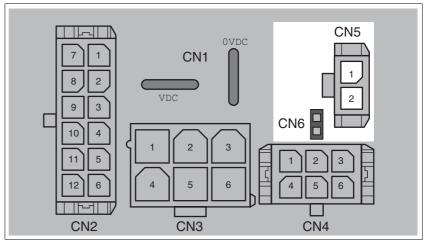
Figure 6.19 Pin assignment of safety function
