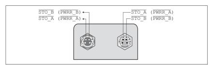
Figure 6.22 Pin assignment
