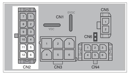
Figure 6.10 Pin assignment of Profibus fieldbus interface
