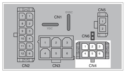
Figure 6.18 Pin assignment of the 24V signal interface
