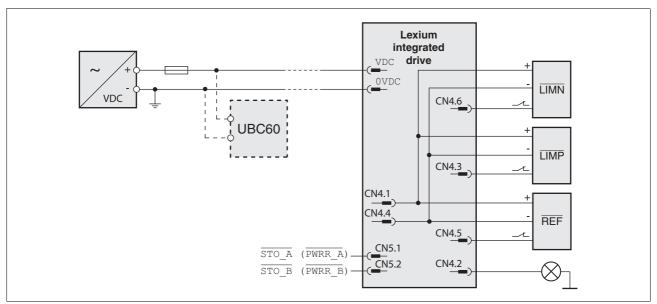
Figure 6.1 Wiring example
