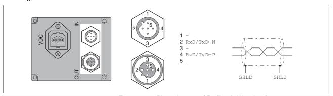
Figure 6.11 Pin assignment of Profibus fieldbus interface
