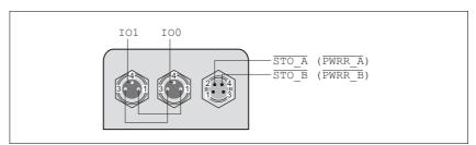
Figure 6.21 Pin assignment
