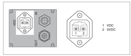
Figure 6.7 Pin assignment supply voltage
