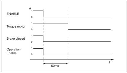
Figure 8.9 Applying the holding brake
