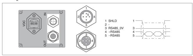
Figure 6.17 Pin assignment of the RS485 fieldbus interface
