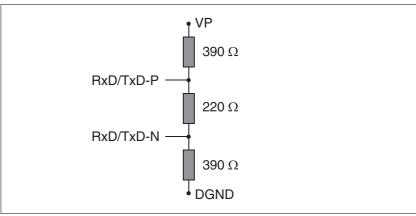
Figure 6.8 Terminating resistor
