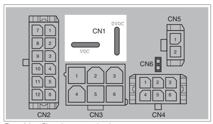
Figure 6.6 Pin assignment supply voltage
