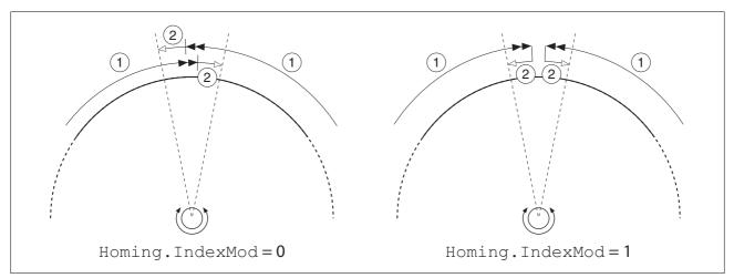
Figure 8.6 Reference movement to index pulse
