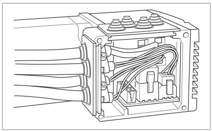
Figure 6.5 Inserting the cable entries
