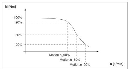
Figure 7.1 Typical torque characteristic of a stepper motor
