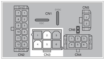
Figure 6.16 Pin assignment RS485
