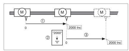
Figure 8.7 Positioning by 4000 increments with position setting
