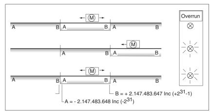
Figure 8.1 Positioning range and range overrun
